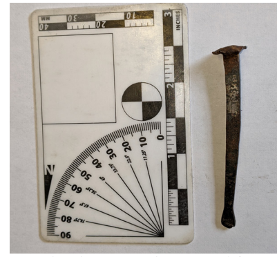
Figure 22 - Chisel point nail extracted from wood ID sample 2
