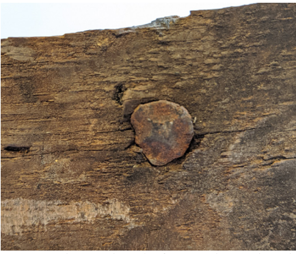
Figure 21 - French rose head of wrought nail embedded in wood ID sample 1
