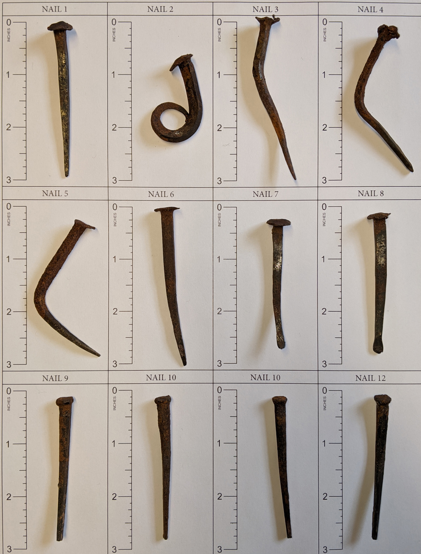
Figure 23 - Nails # 1-12 extracted from roof
