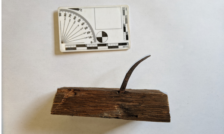
Figure 17 - Wood ID sample 1 with wrought nail embedded
