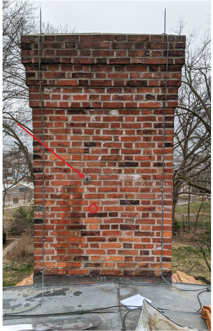
Figure 8 - Southeast chimney with RILEM test location on a mortar joint called out by red arrow and test location on a brick face called out by a red circle
